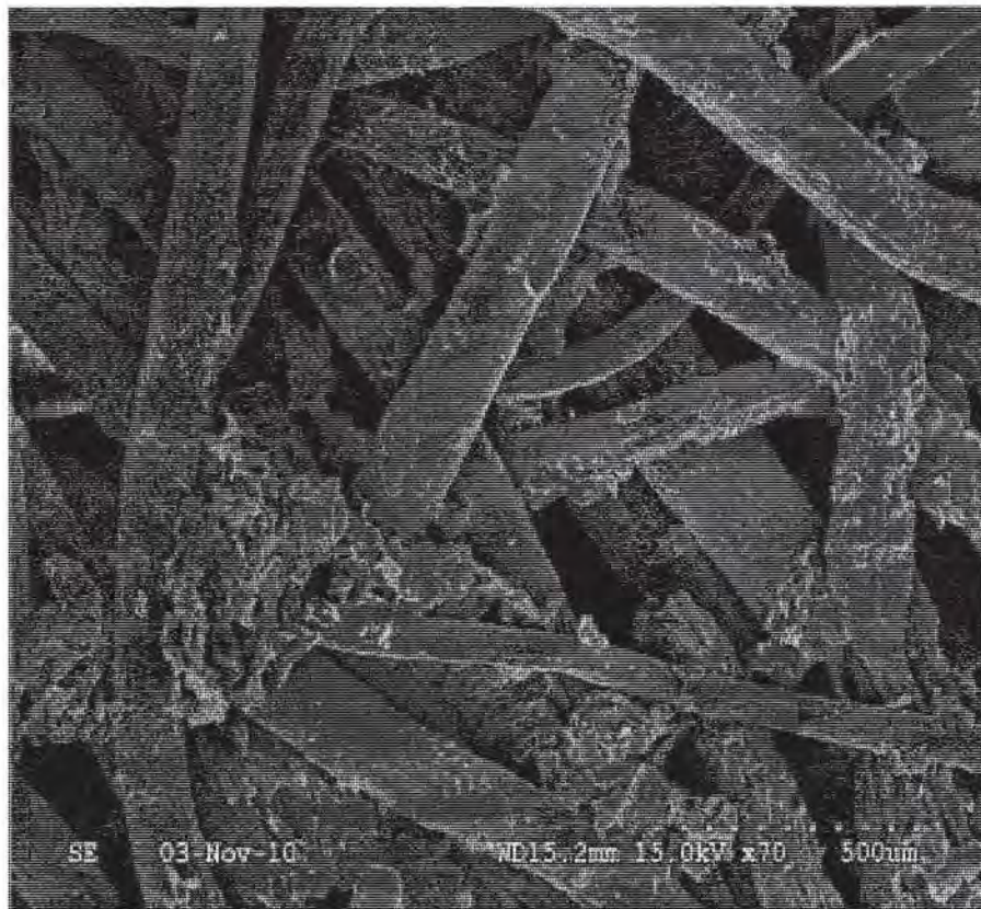
Figure 10. SEM microscopy images of coconut coir (left) and paper + asphalt (right) materials before testing.
