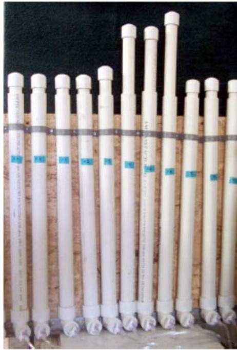
Figure 7. Gas volume totalizers.
